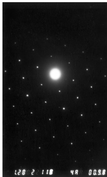
Figure 10 Selected-area diffraction of PMSQ pyrolyzed to 900°C in nitrogen.
